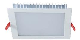
The Orion Mini is a 104 x 104mm low void downlight which uses a Samsung LED engine. The heatsink is constructed from die-cast aluminium complete with aluminium bezel and reflector. The heatsink features spring arms which allows the downlight to be installed with ease.
