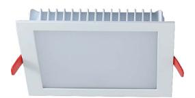
The Atlas is a 140mm diameter low void downlight which uses a Samsung LED engine. The heatsink is constructed from die-cast aluminium complete with aluminium bezel and reflector. The heatsink features spring arms which allows the downlight to be installed with ease.
