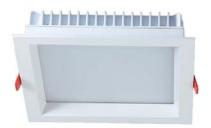
The Orion Deep Mini is a 104 x 104mm low void downlight which uses a Samsung LED engine. The Orion Deep has a 10mm recessed bezel feature for anti-glare cutoff. The heatsink is constructed from die-cast aluminium complete with aluminium bezel and reflector. The heatsink features spring arms which allows the downlight to be installed with ease.
