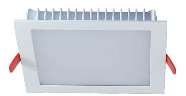
The Orion Max is a 180 x 180mm low void downlight which uses a Samsung LED engine. The heatsink is constructed from die-cast aluminium complete with aluminium bezel and reflector. The heatsink features spring arms which allows the downlight to be installed with ease.
